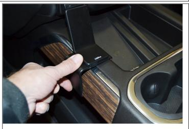
2. Press down on the left side of the ProClip and, at the same time, press to the right on the bottom edge of the ProClip to hook the lower edge of the ProClip under the left side panel of the center console.
