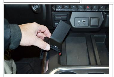
1. Clean the area where the ProClip will attach. The adhesive tape cover must be removed. Place the ProClip in your hand so the ProClip label (sticker) is in an upright position.
